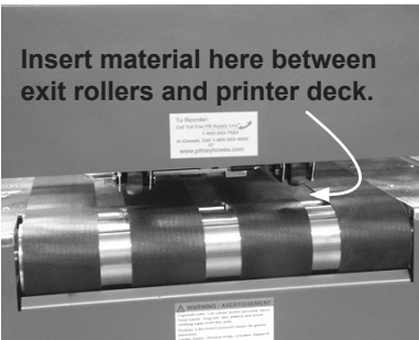
Exit rollers are lifted off of printer deck. Media thickness knob adjusted to thickest setting.
