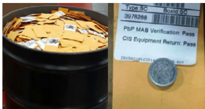
Reusing original packaging to separate the battery terminals, while storing them in mineral oil.
