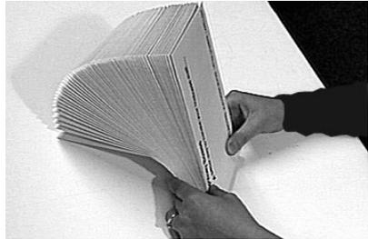
4. Place the stack of envelopes into the feeder with the flap side **UP** and flap **LAST**.
