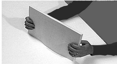
4. Place the paper stack onto the feed deck. Allow the deck to move down and the top of the paper stack to slide under the feed roller.
