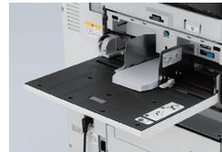
The feed tray, with a thick-paper capacity, allows you to print smoothly on envelopes and other thicker paper.
