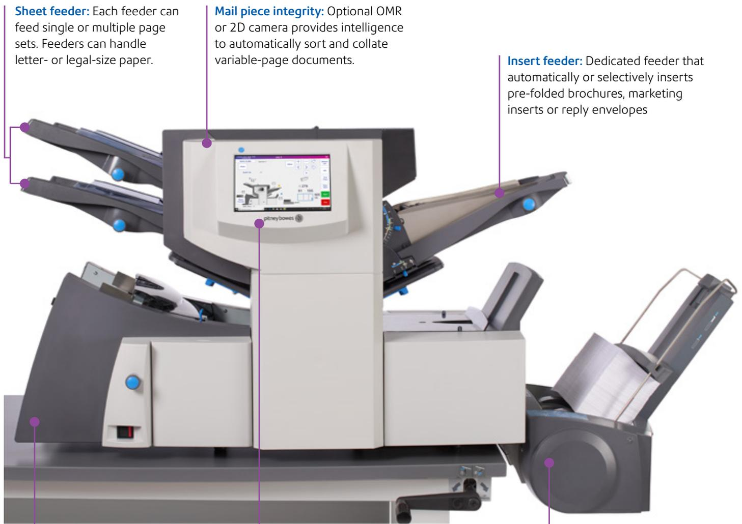
**Sheet feeder:** Each feeder can feed single or multiple page sets. Feeders can handle letter- or legal-size paper.
