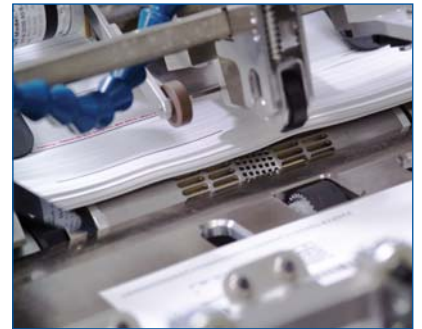
Vacuum-based separation ensures colour forms feed without scuffing
