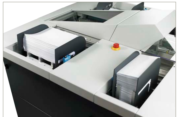
Sheet and insert feeders hold 1,000 and 1,500 items respectively
