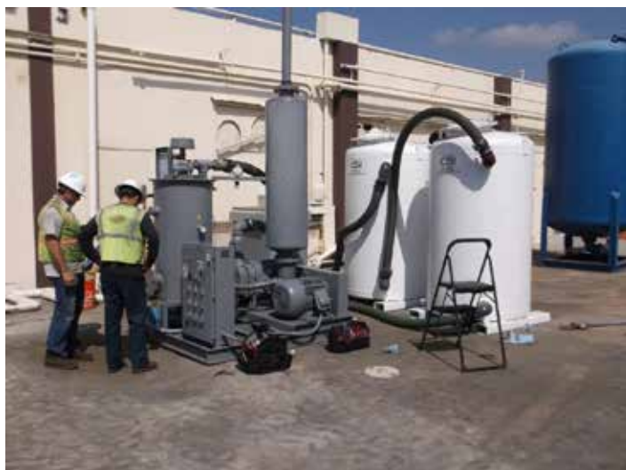
View of interim Soil Vapour Extraction system – former CMI site
