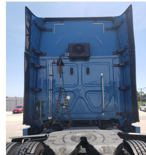
Truck cab with APU to reduce idling emissions.
