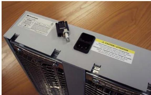
5. Plug in the Dryer AC power cord back into the Stacker and turn the power on. If the blown fuse condition occurs again, call Pitney Bowes for service.
