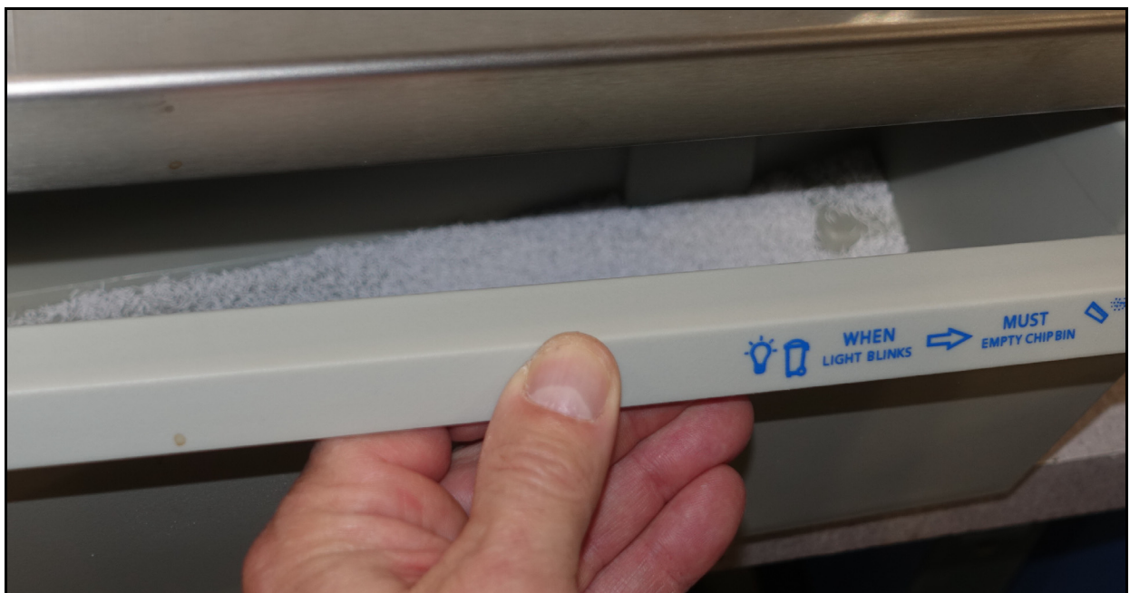
Figure 4-3: Opening the Chip Bin tray
