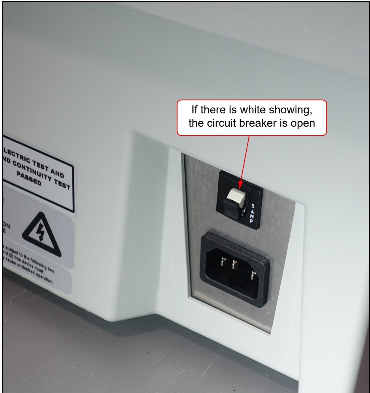
Figure 4-15: Open circuit breaker
