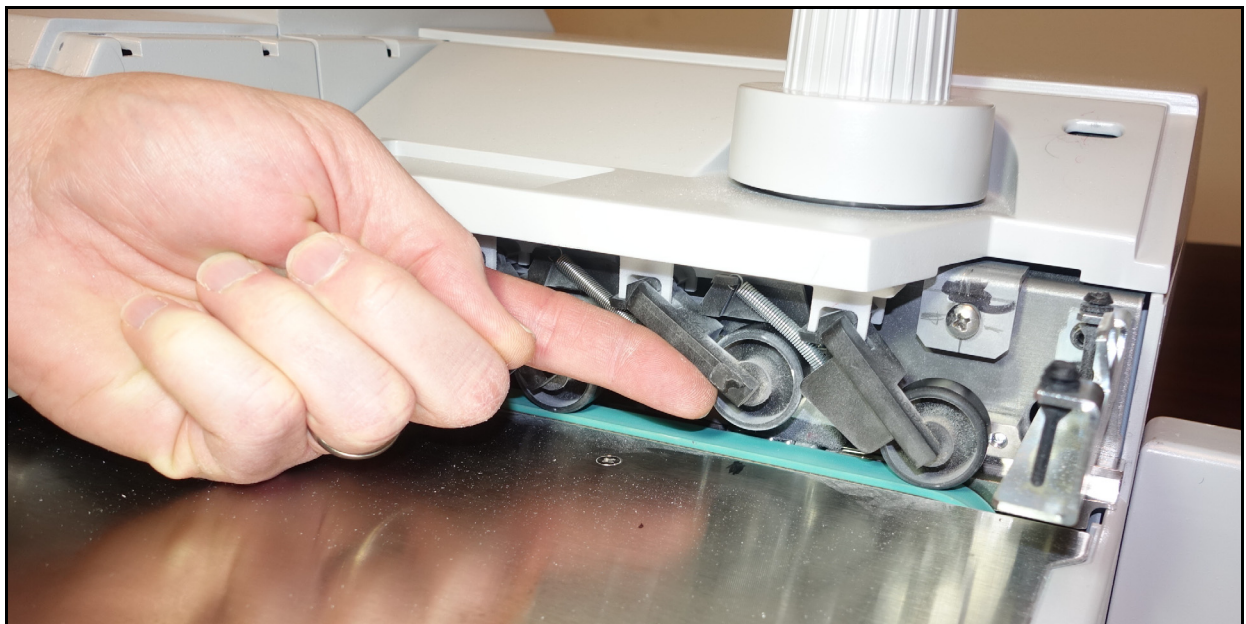
Figure 4-12: Cleaning under the nip wheels
