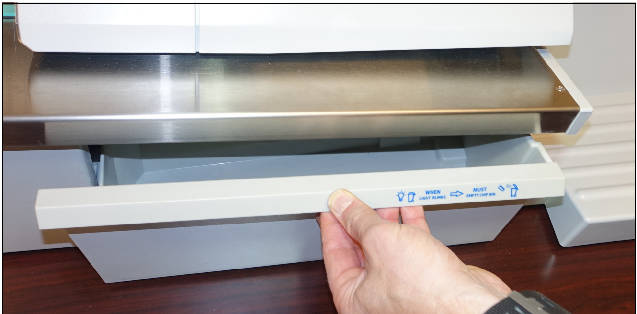
Figure 2-9: Bin tray removal interlock triggering
