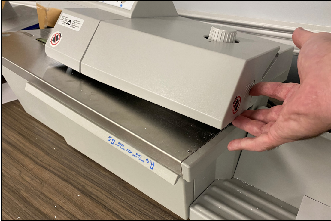
Figure 2-8: Top cover removal interlock triggering
