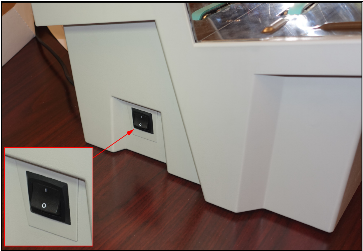
Figure 4-5: AC power switch
