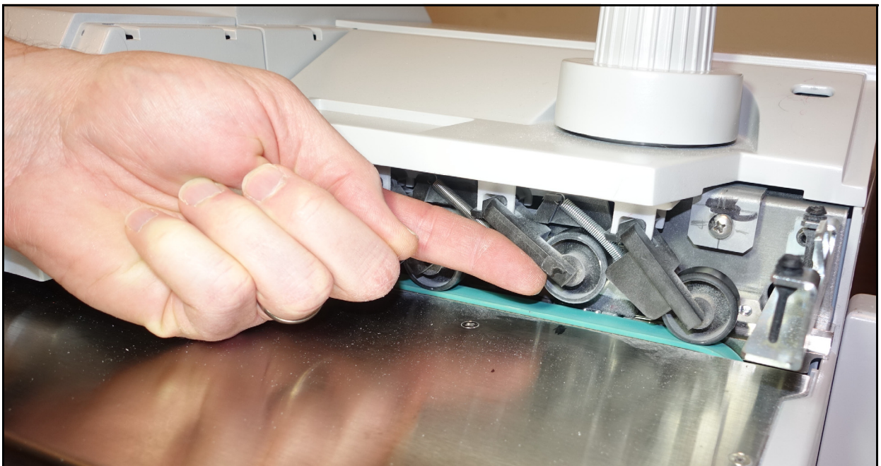
Figure 4-15: Lifting the nip wheels
