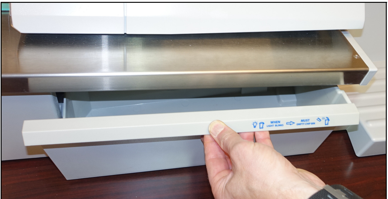
Figure 2-10: Bin tray removal interlock triggering
