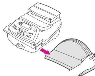
2e. If your meter has a scale, remove it now by lifting straight up and off as shown.
