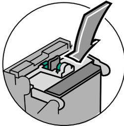
9. Close the top cover. The system automatically recognises the new cartridge and in a few moments returns you to the Home screen.
