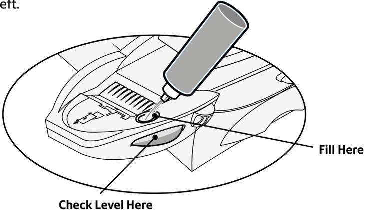
2. Add enough sealing solution or water to bring the sealant level up to the bottom of the fill hole. We recommend sealing solution because it helps keep your moistener clean and improves sealing efficiency.
