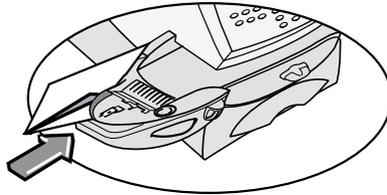
3. Position the envelope or tape sheet against the registration wall of the system and slide it to the right until the system grasps it. The system prints the digital meter stamp and ejects the envelope/tape sheet.
