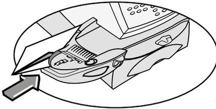
4. Slide the envelope to the right until the system takes hold of it. The system seals and ejects the piece.
