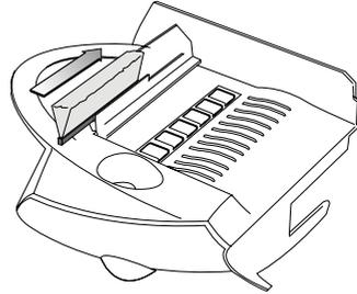
8. If you need to clean the wick and holder, continue with Removing the Holder and Wick procedure on the next page. Otherwise, push down on the blue release lever on the moistener.
