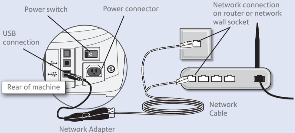
Plug the power cord into a convenient outlet and into the machine. Turn the power switch ON.
