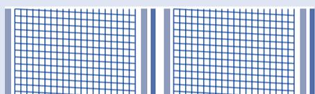
**Good print** - no broken lines in the centre of the test print
