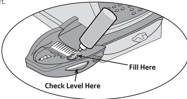
2. Add enough sealing solution or water to bring the sealant level up to the bottom of the fill hole. We recommend sealing solution because it helps keep your moistener clean and improves sealing efficiency.
