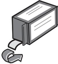
6. Lower the ink cartridge into the cavity. The ridges on either side of the cartridge will slide into the grooves.
