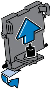
7. Squeeze the two gray tabs on either side of the new print head and slightly angle the print head while sliding it back into its holder.
