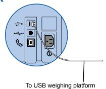
If you have purchased an external USB weighing platform, connect it to the back of the DM300c using the USB cable supplied.
