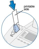
Load tape into tape feeder and press Tape button.
