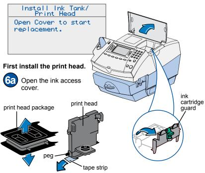
Remove the print head from packaging and remove tape strip.
