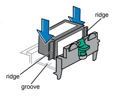
Remove the ink cartridge from the bag and make sure the tape strip is peeled off.
