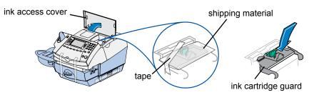
Open ink access cover and remove tape and shipping material. Then close ink cartridge guard followed by ink access cover.
