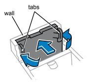
Squeeze the tabs on the sides of the print head and push the print head flush against the wall.
