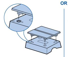
Assemble weighing platform.
