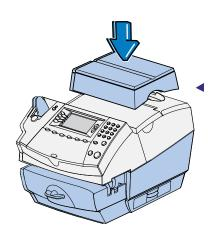
Install the assembled weighing platform on the system.
