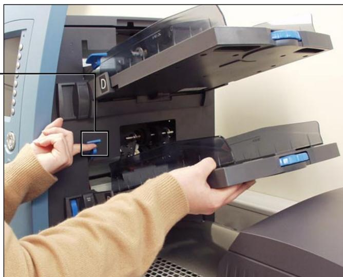
Figure 3.1.1: Lift the Separator and slide the Tray into the tray mounts.
