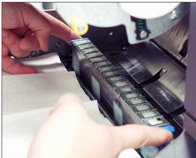
**Figure 5.3: Removing the Old Wick Cartridge**
