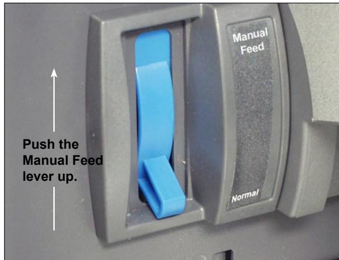
Figure 2.4: Manual Feed Lever.
