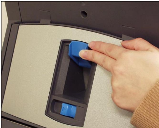
Figure 3.8.1: Push up on the Separator Gap Lever
