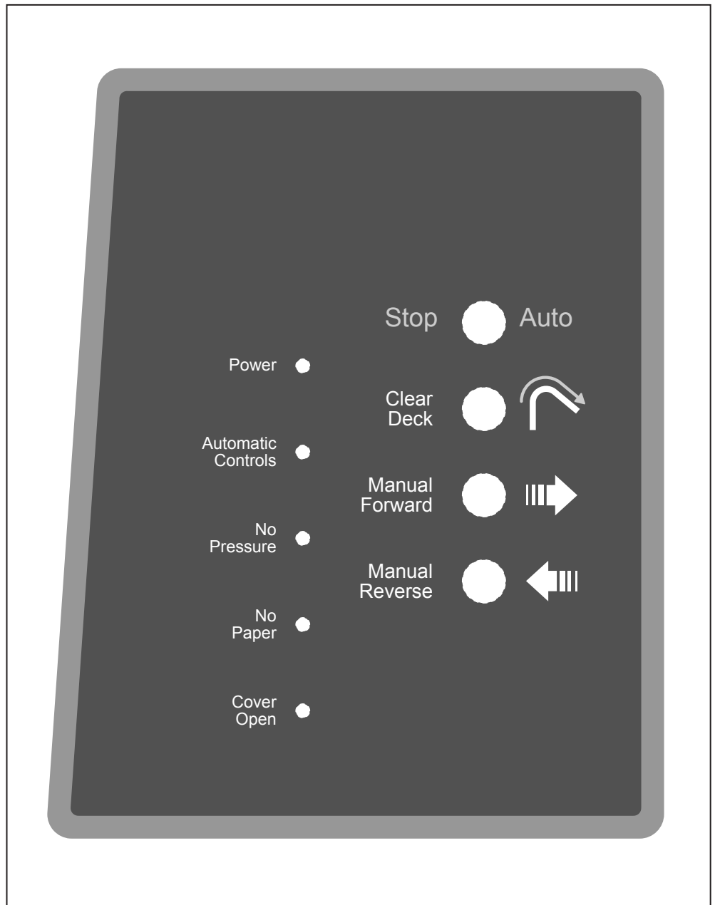
F734/F735 High Capacity Feeder Control Panel
