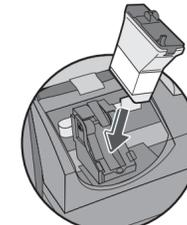
4. Insert the new ink cartridge. Insert the base of the cartridge first before pushing the top back.
