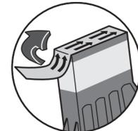
3. Open the packaging for the new ink cartridge and take off the protective tape from the bottom.
