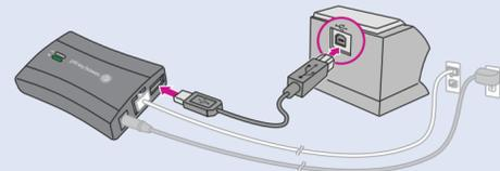
4. Now connect the franking machine to a power outlet. Startup screens appear and you will hear noises as the franking machine initialises.
