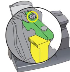
2. When prompted, lift the top cover and press the unlock symbol on the cartridge latch. Remove and discard the yellow packaging material.
