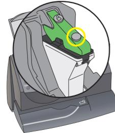
5. Press the ink cartridge latch down until it clicks and holds the cartridge in place.
