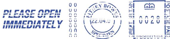
The illustration above shows a bad print with missing lines. Only approved ink should be used in the machine.
