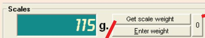
To re-zero the platform, click on the **0** button with nothing on the scale platform.
