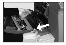
Push the rollers firmly down until they latch into position.
