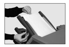
Take the stack of paper and aerate (fan) it to ensure that individual sheets are not stuck together.
