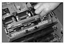
Install the four new felts into the sealer tank. They will only fit one way. Make sure to push them fully down into the tank.
