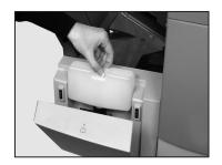
**Note:** If the sealer unit was completely empty, allow time for the fresh solution or water to soak through the sealer *before* you resume operation. This helps assure a good seal.
