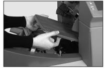
release them. Slide the plate into its location guides and release the catches to lock the plate in position.
