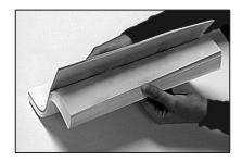
Jog the stack back into alignment. The sheet feeders take the paper stack aligned in a manner similar to that used for a photocopier paper cassette.
