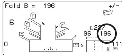
If you are programming an inserting job, the setting Envelope Depth will now appear. If you are programming a fold only job, the display will jump straight to the 'Confirming the Job Setup' section on page 2-20.
