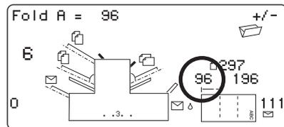
If you want to change the 'standard' setting, press **Change (+/-)** until the length of fold required is displayed. The symbol | — | shows the fold panel you are adjusting.
