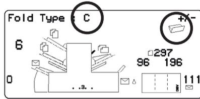
**Note:** For OMR scanning jobs, **DO NOT** manually change the automatically set fold length dimensions for 'Fold A' and 'Fold B'
