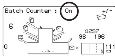
If Batch Counter is turned On, the machine will now request the batch quantity. The default quantity is 50, but you may select any value up to 999 using the **Change (+/-)** buttons.
