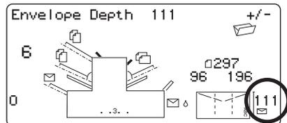
When the envelope depth is set as required, press **Next (▶)** to advance to the next setting...
