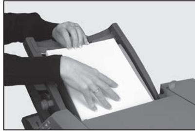
**Note:** When using both Sheet Feeders with accordion fold, Sheet Feeder 2 must be used for the prime (address bearing) document.
