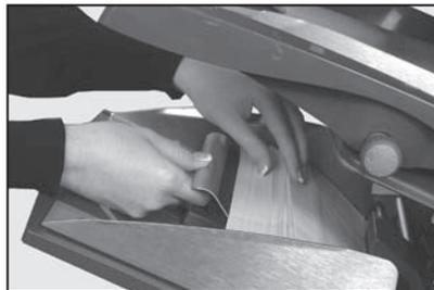
Let the 'wedge' slide down behind the stack so that the envelopes are supported.
