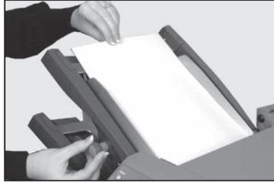
2. Take the stack of paper and aerate it to ensure the individual sheets are not stuck together.
