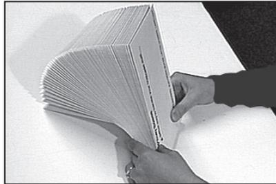
3. Place them on the feed deck with the flaps up and trailing. **The lead edge of the first envelope should be under the front feed roller and the stack of envelopes should be 'shingled' on the deck as shown.**
