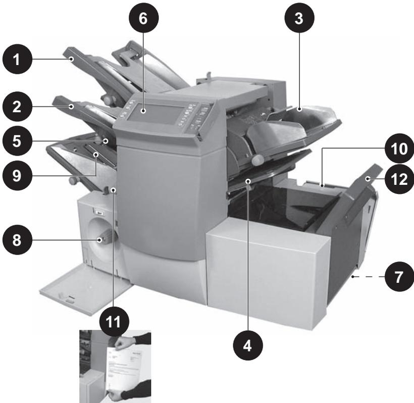
**1 Sheet Feeder 1** This feeder is intended for feeding material that requires folding.
