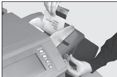
2. Refer to the 'label' located on the Insert Feeder. Compare your insert with the diagram. Read off the settings for the Insert Feeder blue lever (numbers 1 to 9) and the separator shield (letters A to D).
