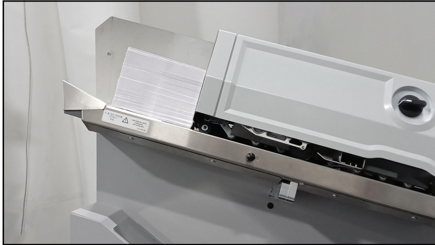
Figure 5-6: Mail positioned in feeder
