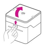
Press up on the latch to open the cover.
