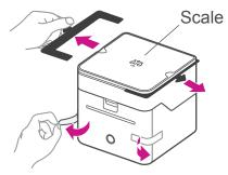
Remove the protective scale spacers and tapes.
