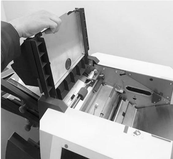
3. Remove the jammed material from the accumulation area.
