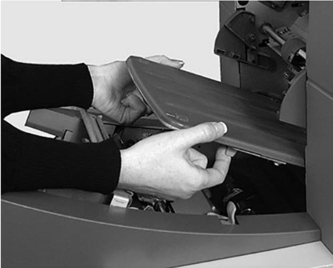
2. Remove the jammed material. If necessary, *use the manual advance knob* to move the material forward.
