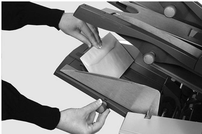
3. Aerate and fan the stack of envelopes so the individual envelopes are not stuck together.
