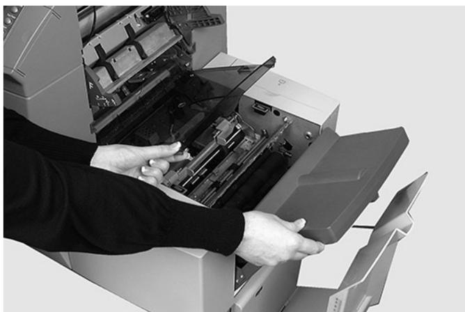
2. The points identified here can be unlatched to allow access to jammed material.
