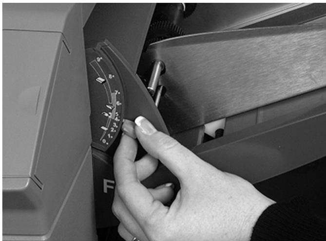
5. Set the blue separator shield lever to the letter required.
