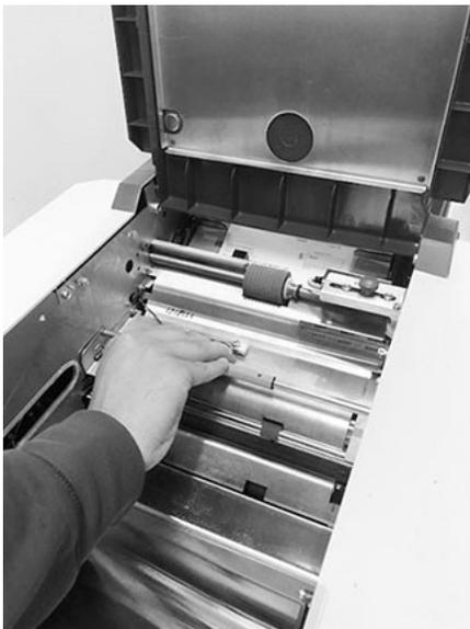
5. Pivot the guide bar back into place using the blue handle; be sure it clicks into place.
