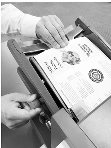
2. Aerate (fan) the stack of paper to ensure that individual sheets are not stuck together.
