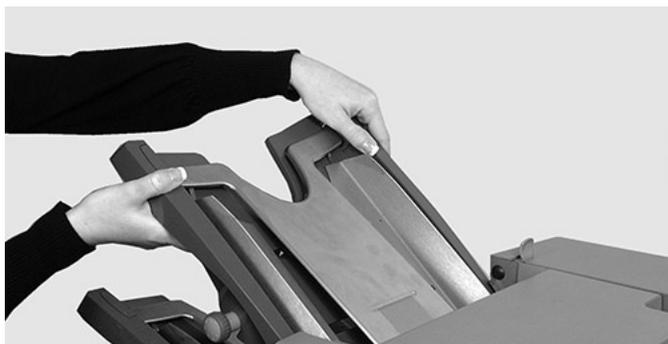
2. Remove the jammed material. If necessary, *use the manual advance knob* to move the material forward.
