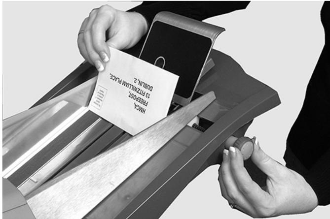
2. Once the guides are touching both sides of the insert, turn the adjustment knob 1/4-turn in the opposite direction. This sets the correct clearance between the guides and the insert.
