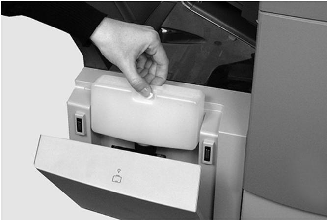
3. Fill the bottle with the solution to the level indicated.
