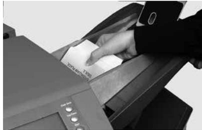
7. Let the wedge (material prop) slide down behind the stack to support the inserts.
