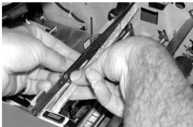
7. Using the plastic tweezers provided in the kit, remove all four felts from the sealer tank. Discard these old felts.
