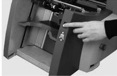
2. Use the side guide adjustment knob to adjust the side guides to the *width* of the envelopes. Once adjusted, back-off the adjustment knob 1/4 turn.
