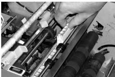
9. Push down on the blue tab to return the upper felt assembly to its operating position. Make sure that the blue latches (A) spring out and fully latch into position.
