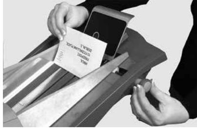
2. Refer to the labels located on the insert feeder and match your insert type (slip, reply envelope, pre-folded, booklet) with the icon and color.
