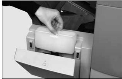
*NOTE: If the sealer unit was completely empty, allow time for the fresh solution or water to soak through the sealer before you resume operation. This helps assure a good seal.*
