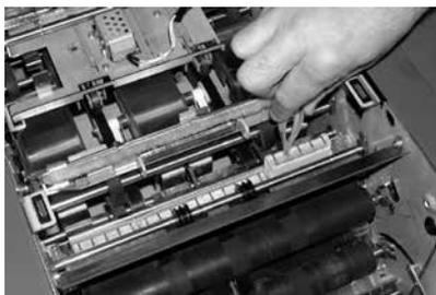
8. Install the four new felts into the sealer tank. They will only fit one way. Push them fully down into the tank.
