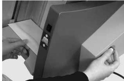
3. Take the stack of envelopes; aerate and fan it to ensure that individual envelopes are not stuck together.
