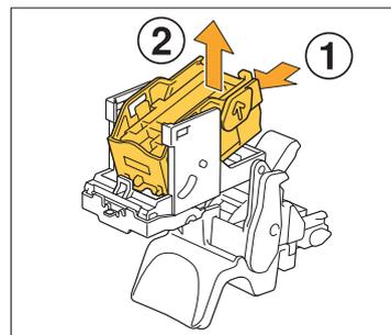
**7** Insert the front part of the new staple case into the cartridge, and then insert the back part.
