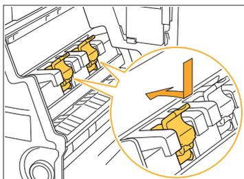
Be sure to install the staple cartridge to the position aligned with the ▲ mark of the booklet unit.
