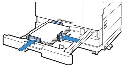
The machine detects the size of the paper based on the stopper position. Make sure to position the stopper against the edge of the paper.
