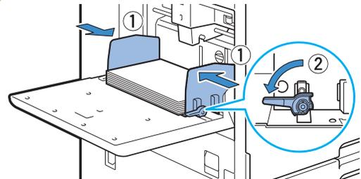
The machine detects the paper size based on the guide position. Make sure to position the guides against the edges of the paper.
