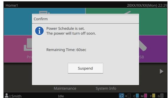
If you do not want the machine to turn off, touch [Suspend]. Close the [Confirm] screen to suspend the power-off process. The [Confirm] screen will be displayed again after one minute.
