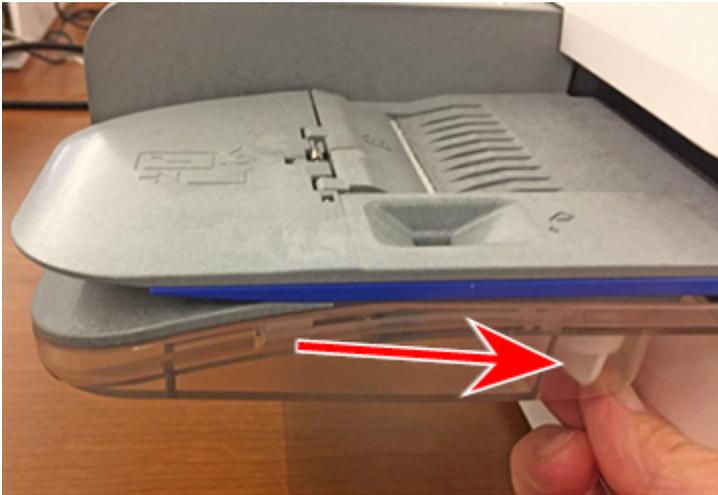
2. Lift the moistener brush assembly off the top of the moistener base.
