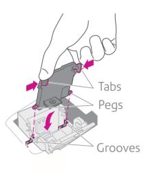
d. Squeeze the tabs and slide the Printhead pegs into the lower set of grooves.
