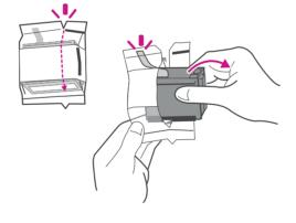
e. Keep squeezing the tabs and push the Printhead flat against the and make sure you remove the wall. The tabs will click open when silver foil strip. placed correctly.
