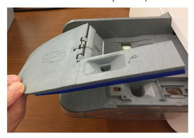
3. Turn the assembly over and slide the moistener brush out of the holder.
