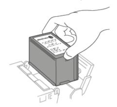
7. Squeeze the tabs on either side of the printhead.
