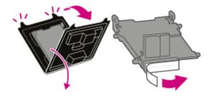
5. Squeeze the tabs and slide the printhead pegs into the lower set of grooves. **Important:** This step is critical to prevent device damage.
