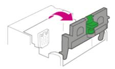
4. Unwrap the printhead and remove the protective strip.
