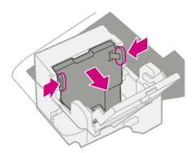
8. While squeezing, lift and tilt to the printhead to the right. The printhead should come up out of the device.
