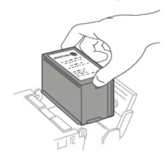
7. Squeeze the two gray tabs on either side of the printhead.
