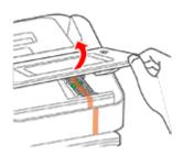
2. Remove the packing tape from the ink carriage.
