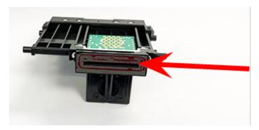
10. Squeeze the tabs and slide the printhead pegs into the lower set of grooves.
