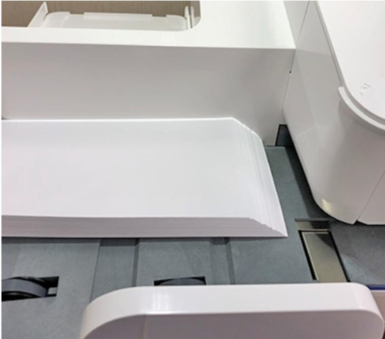
3. Slide the side guide up to the mail stack. Leave about 1/8" space (about the thickness of 2 quarters) between the stack and the side guide so the envelopes do not drag against the guide.
