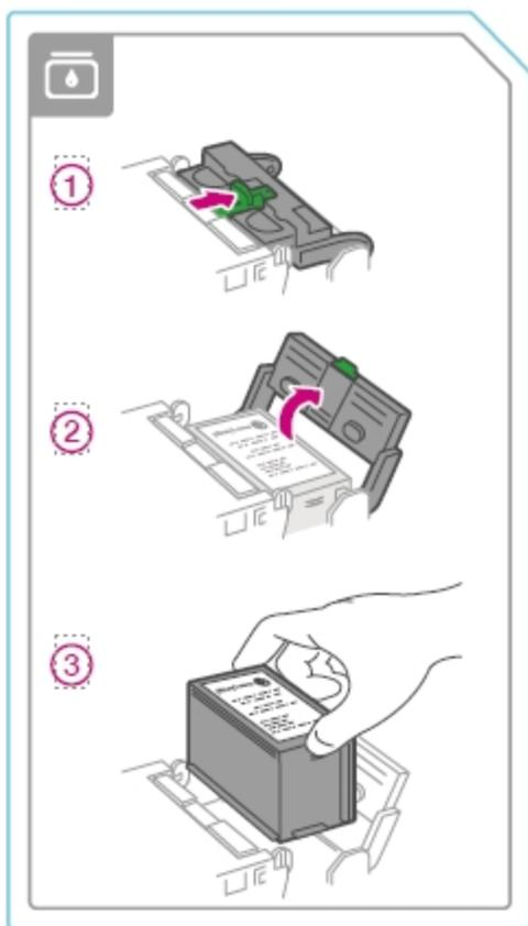
6. Insert the new ink cartridge, then close the ink cartridge guard.
