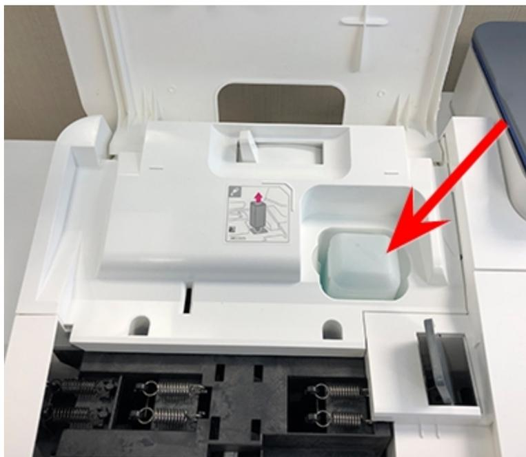
3. Remove the moistener bottle and place it with the cap up on a flat surface.
