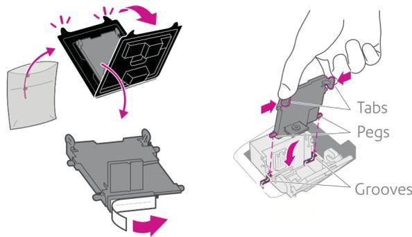
c. Unwrap the printhead and remove the protective strip.
