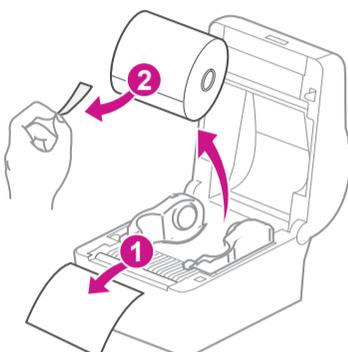
3. Install the label roll and feed the label through the media guide.
