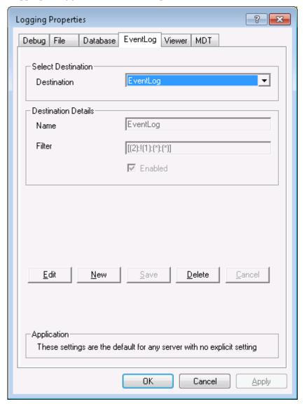
Select the "EventLog" tab of the "Logging Properties" dialog. The Filter value should be set to [(2):!(1):(\*):]. This setting is usually enabled by default.
