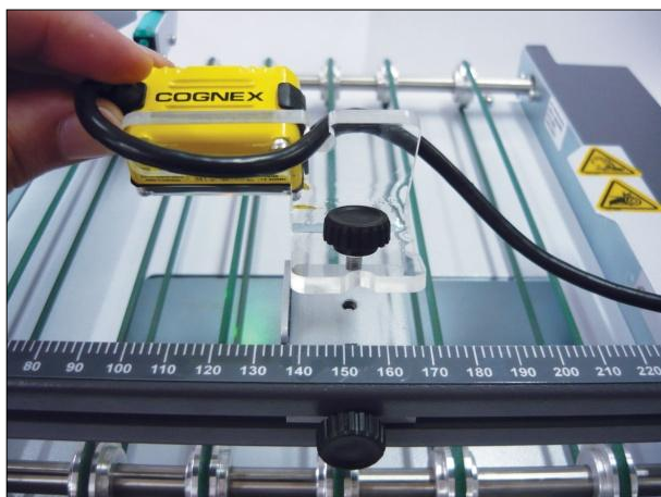
Figure 30 – Changing Camera Bracket Orientation
