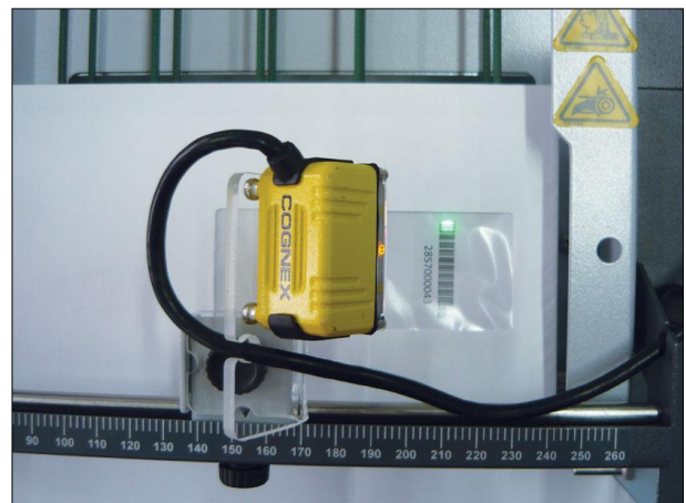
Figure 29 – Camera Orientation According to Code Orientation
