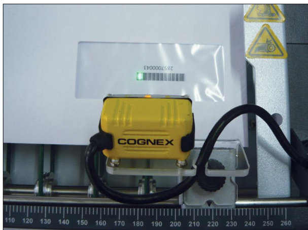
Figure 29 – Camera Orientation According to Code Orientation
